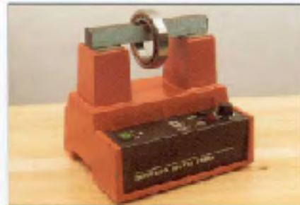
*Use an induction heater for assembly (or arbor press for interference fits).*
