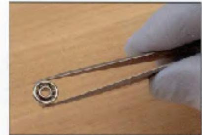
*Use tweezers to install miniature and instrument bearings.*
